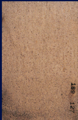
Galvalume test panel shows only moderate edge discoloration after 23 years in same rural environment.
